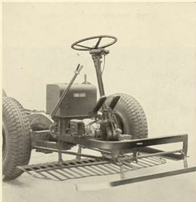
Chassis at driver's end showing controls.
