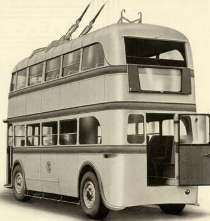
Rear View of Trolley Bus, showing emergency exits open.
